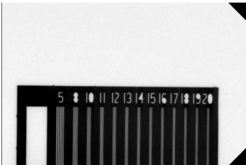
Figure 7 - Resolution test strip placed directly on the Hamamatsu detector. The test strip is placed vertically, but the line pairs are horizontal along the detector.
